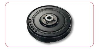
Transmission of crankshaft vibrations to ancillary units can produce an increased noise level, severe wear of adjoining components and undesirable vehicle vibration. The decoupled belt pulley is specially designed to meet the requirements of modern, high performance diesel engines, which develop a considerably higher vibration response than petrol engines.
